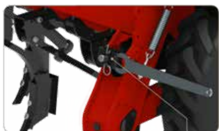
Mounted version (Standard). Seeding depth is adjusted mechanically.
