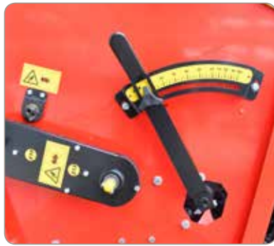
Step-less CVT gearbox with seeding rate test handle.
