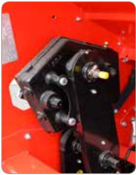
Step-less CVT gearbox with seeding rate test handle.
