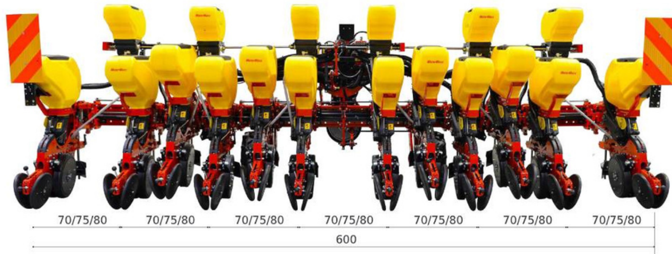
Version: 8 rows, 70/75/80 cm row spacing, 6 m working width
