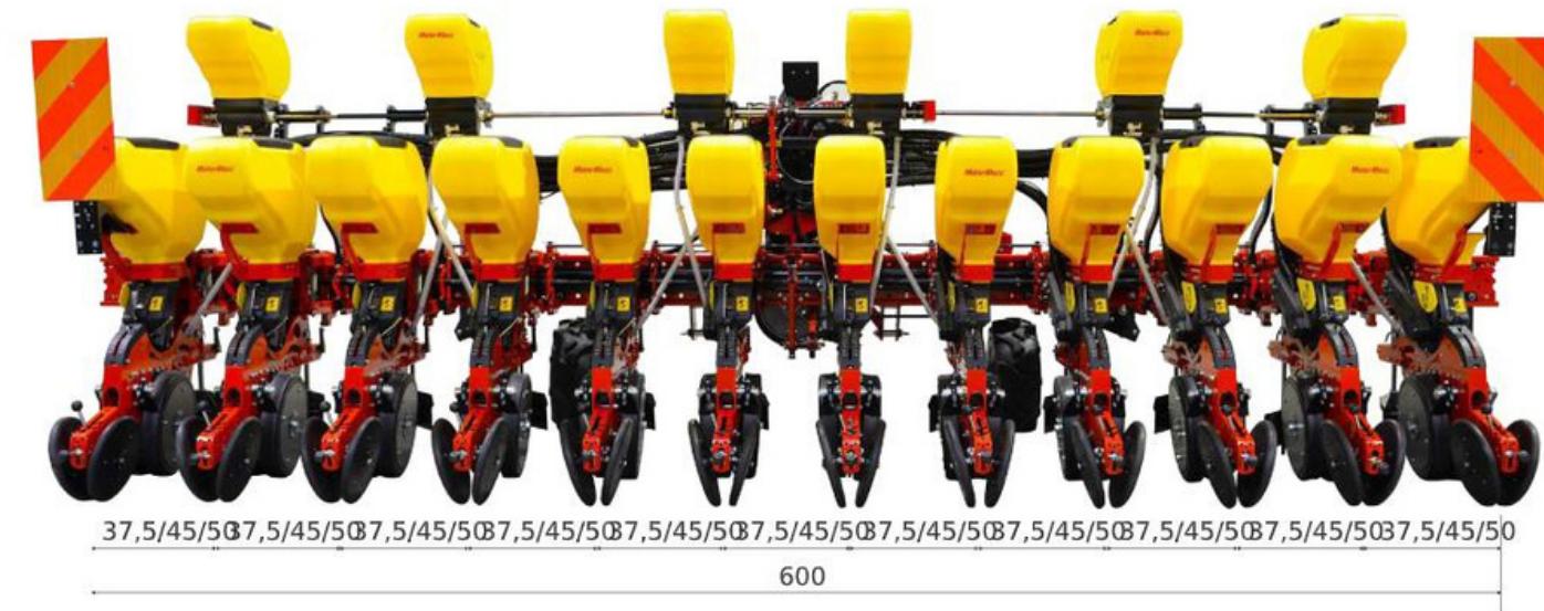
Version: 12 rows, 37,5/45/50 cm row spacing, 6 m working width
