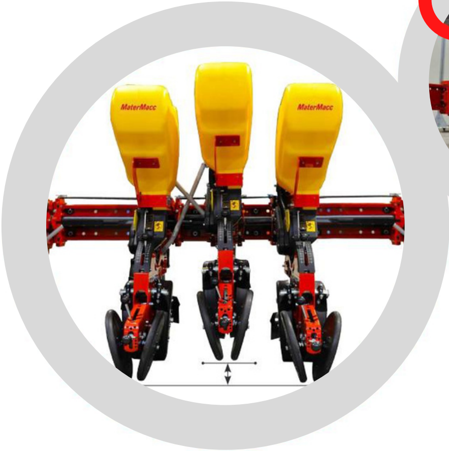
Version: 8 rows, 70/75/80 cm row spacing, 6 m working width
